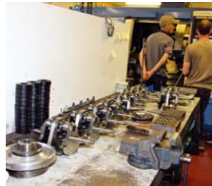
Clockwise from below: crankshafts are made in batches of 40; each crank starts as a 70kg piece of billet and ends up 8.2kg; big-port heads awaiting over-size valves; donor heads awaiting modification; Seeley frame meets Commando engine; Maney-Commando powerplant.
